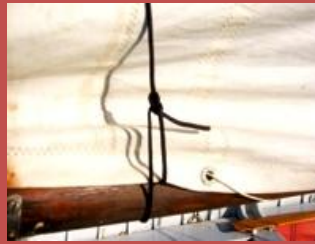
Picture 6: Bowline tied around the boom
